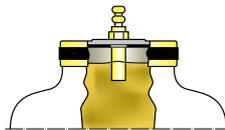
The extended nozzle of the plug must be immersed in the fluid to avoid sprays or air and oil emulsions.
