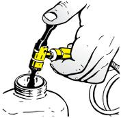
Before bleeding it is important to fill the brake fluid reservoir by means of the brake bleeder quick-release connector.
