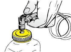
Connect the brake bleeding device to the reservoir by means of the quick-release connector.
