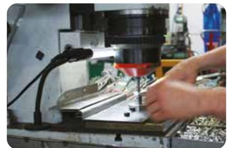
The very slim design with a diameter of only 25 mm makes it possible to illuminate even hard to reach compact areas.
