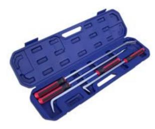
Chrome Molybdenum 16mm steel shafts with satin chrome finish and textured handles Contents : 900mm (straight) - 900mm (45°) - 600mm (75°) - 600mm (90°) Supplied in plastic storage case
