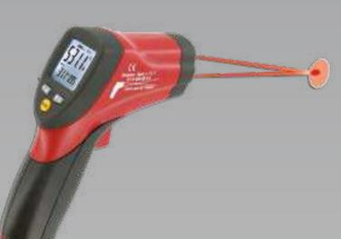
Precise non-contact thermometer Two laser points to a single spot when the unit is at the optimal distance from the target Temperature range : -50°C to 550°C Unit selectable (C°/F°) Accuracy : +/-2% Distance ratio : 12:1 Emissivity adjustable Ideal for air-conditioning, cylinder temperature, brake temperature, cooling system temperature Batteries included Automatic Data Hold Set high and low alarms Trigger lock
