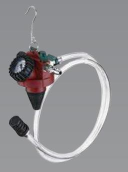
Purge trapped air from cooling system to eliminate the possibility of engine damage due to overheating Performs vacuum leak test on cooling system Refills cooling system free of trapped air quickly, efficiently and with no mess Universal rubber body covers most vehicle radiators Muffler dampens noise output during operation Working pressure: 5~8 bars Max pressure: 8 bars Air consumption: 165L/min Inlet: 1/4 bsp
