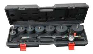
Delivered with 8 conical caps from 35mm to 90mm Caps with rugged surface for a better grip in the tubes Includes a gauge with integrated regulator for a better leaks reading Allows the technician to pressurize the whole turbo and inlet system in order to detect quickly and accurately potential leaks
