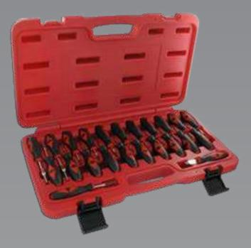
A comprehensive terminal tool set that incorporates up to the minute products for use on standard terminals and vehicle computer connectors Includes special tools for coolant sensors, wiring harnesses and terminal blocks on Chrysler, Hyundai, Kia and Mitsubishi vehicles
