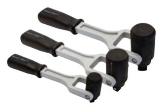
Loosen rusted or frozen bolts with high impact force Produces 8 x torque multiplication with each hammer blow No compressed air required for operation **Precision impact** Bi-directional - use to loosen and tighten fasteners Swivel head aids with operation in limited access situations Swivel head allows speed brace action to spin fasteners off after initial loosening Impact absorbing composite handle Use with impact sockets and driver bits
