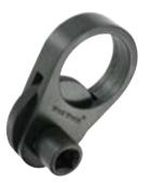
Use on steering racks to service inner tie rod ends, directly on the vehicle NEW larger size to provide coverage for domestic and import light trucks and SUV's Diameter 38mm to 48mm
