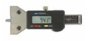
Allows to check tyre wear, brake shoe... From 0 to 25mm Resolution: 0.01mm LCD display Zero setting at any position Quick and efficient reading Metric/inch system interchange
