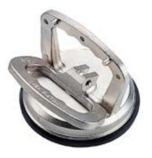
Ideal for carrying glass, marble, furniture and domestic appliances One-hand operation : make vacuum by joining the two handles Diameter : 123mm Loading capacity : 40kg (GS : 15kg)
