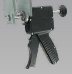
A lot of modern cars are mounted with electrical hand brakes. The AB70915 is the ideal tool to push back the pistons of those type of brakes. Fast and easy to use Powerful : generates over 215kg of force Universal adapter : fit single, twin or quad piston Prevents damage to pistons, seals or calipers (no pliers, no screwdrivers) All pistons are retracted at the same time - no piston getting out
