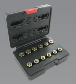
Used in association with HU35026, this set will allow to close injectors fuel inlet directly on the common rail. The purpose of this operation is to identify if an injector is leaking or not Works for 3, 4, 5 and 6 cylinders engines Kit includes 6x M12x150 plugs and 6x M14x150 plugs
