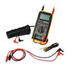
Specially designed for all automotive applications Automatically turns off after 10 min Accessories: test and temperature probes, test clamps, inductive clamp for tachometer FUNCTIONS: Voltage : AC (3,2V - 1000V) DC (3,2V - 750V) Current : AC (32mA - 10A) DC (32mA - 300mA) Resistance from 320Ω to 320KΩ Frequency from 0,01Hz to 32kHz Diode check RPM from 0 to 12,000 Temp. measurement (-20°C - +1370°C)
