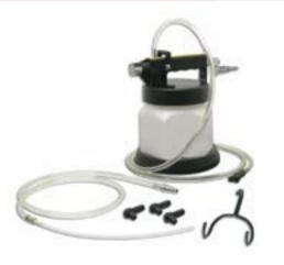
High quality, professional unit Allows clean, quick fluid evacuation Variable thumb throttle holds desired flow rate Includes 3 semi-rigid probes with various diameters + 1 brake bleeding tube Compressed air operation Integrated 1.8 litre capacity fluid collection reservoir Quick-disconnect coupler for accessories Quiet, muffled exhaust Automatic overflow prevention
