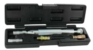
Have you ever tried to force grease through a grease joint and couldn't? Now you can! The patented Grease Joint Rejuvenator® forces light oil into a grease joint, flushing out old hardened grease and allowing new grease to be pushed through.
