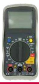
MEASURES: Voltage DC : 600V Voltage AC : 600V Current DC : 10A Current AC : 10A Resistance : 20M  $\Omega$ Diode check : test current of 1mA maximum, open circuit voltage 2.8V DC typical Continuity test : audible signal will sound if the resistance is less than approximately 30 $\Omega$ Temperature: from -20°C to 760°C
