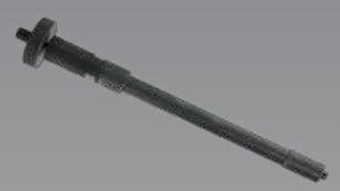
Removes stuck copper injector base seals Adjusts easily to inner diameters from 6,40 to 9,50mm Adjustable depth of the expandable collet Usually used in conjunction with HU41004 seat cutter set
