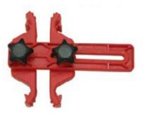
Holds valve timing on overhead cam engines during timing belt service Suits timing gear diameters from 101 to 152mm Suits gear spacing from 1.6 to 76mm Patented 'Uni-fit' tooth design suits a large range of cam gear sizes Patented friction locking system allows infinite locking positions to suit most cam gear configurations
