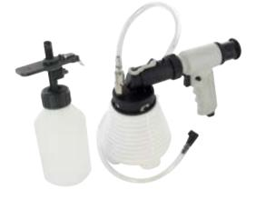
Uses compressed air to generate deep vacuum to bleed old fluid and air rom hydraulic brake system Auto refill unit maintains correct fluid level during bleeding process Reduces repair times increasing productivity and profit New design with unique patented built in safety valves to prevent accidental fluid spray and spillage
