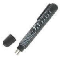
Integrated circuitry checks moisture content of fluid by measuring the electrical resistance and comparing it with acceptable limits Easy calibration check using water 3 LED read-out (green = < 1.5% ok / yellow = from 1.5% to 3% / red = >3% wrong) Red LED warns when low battery Battery 1.5V AAA included
