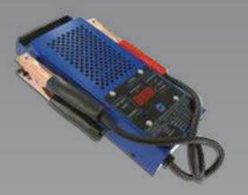
Bright LED digital display Easy to use : push one button to complete the test within 10 seconds Tests 12V battery ratings of 200 to 1000CCA range Tests 12 volt charging system and starter motor system
