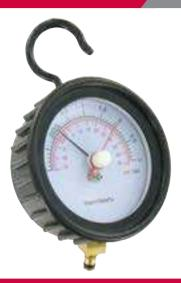
From -1Bar to +3Bar To be used in conjunction with Mityvac pump MI8550 (quick connection) Allows to control the maximum pressure of the turbo during a road test Features a red needle that indicates the maximum pressure reached during the measuring
