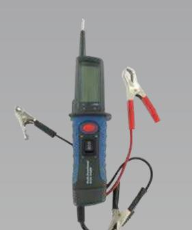
Detects currents from 0V to 24V DC Activate the components with positive or negative current thanks to its 6m cable Determine the polarity and circuit circumstance (short-open / green or red LED) Short cicuit protection Test the continuity of the circuit Locate missing cylinders Measures high tension frequency of ignition system Audible warning Digital LCD display Integrated LED light, ideal for work in dark places Se branche sur la batterie du véhicule Ignition in kV
