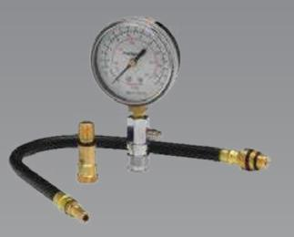
Excessively high or low readings, or compression readings exceeding manufacturer 's specifications from cylinder to cylinder, may indicate an internal engine problem. UNIT FEATURES: 0-300 p.s.i. (0-21 Bars) test gauge Hose assembly with replaceable check valve core 14mm long reach adapter
