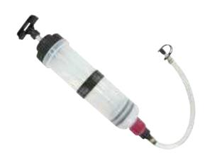
Transparent design to visualise the fluid Suitable for fluid suction and supply in vehicle service Designed for transmission fluid, gear oil and engine oil (not ATF) Features cap to avoid dripping Rotative switch off CAPACITY : 0,9kg / 1,5L capacity
