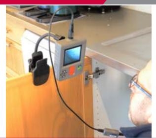
Attach behind the videoscope thanks to its threaded fastener Flexible support (30cm) Powerful grip with antiscratch foam
