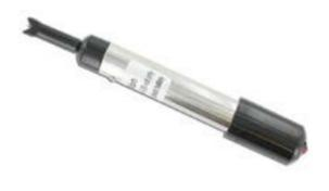
Suitable for testing DC circuits with voltage from 3 and 28V No ground wire or clip required Tester illuminates LED, buzzes and vibrates on contacting live wire Computer-safe for use around delicate engine management systems Supplied fitted with 2 X long life alkaline batteries
