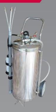
To retrieve fuel following a filling error (gasoline instead of diesel, etc.), remove a submerged fuel pump, change or check the fuel gauge, rinse the fuel tank, during body work, etc. Operates off workshop compressed air (no risk of sparks)
