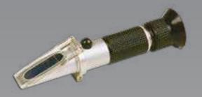
To check: Coolant : from 0 to -50°C Battery : from 1.1 to 1.4Kg/L Windscreen cleaner : from 0 to -40°C AD Blue separated scale from 30 to 35% Plastic model (HU404) and metal model (HU414)
