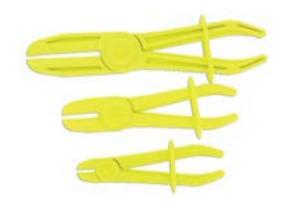
Ideal for flexible brake, fuel and coolant lines (seals heater and radiator hoses) Light weight, non conductive highly visible material Quick and easy to use SET INCLUDES: AB70035: 1 small clamp for diameters < 13mm AB70533: 1 medium clamp for diameters 13-19mm AB70684: 1 large clamp for diameter 19-57mm Clamps can be sold separately.
