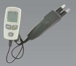
Ideal to diagnose current leaks (consumption) Maximum measuring voltage: 48V, max current: 80A Large LCD display with bar graph Peak hold and data hold function Zero setting for accurate measurement For large, standard and mini blade type fuses
