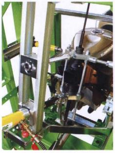
The only and unique system to firmly anchor the frames of motorcycles and scooters, thanks to universal jigs, columns adjustable in height and sliding crossbeams.
