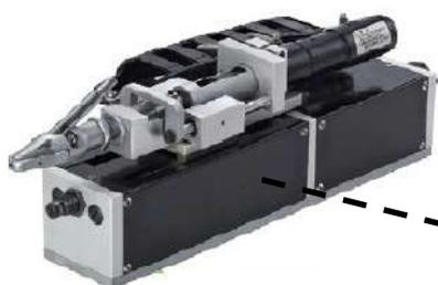
Double stroke feeding and tightening unit
