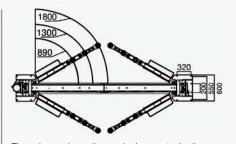
Through experience the required concrete depth (foundation requirement of 250 mm) should be met, this must be checked by the customer. If in exceptional cases the foundation requirement is not met, we offer on page 31 a special solution, which can be used with a concrete thickness of 200 mm to 250 mm
